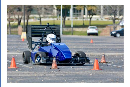
F20 drove with all of the aerodynamics package installed. When we began testing we chose to wait on the wings so that we could focus on other areas of the car. At the end of Spring Break we graduated to having the full aerodynamic package on the vehicle, and although we have yet to gather much data the car looked fantastic going around our test track!
