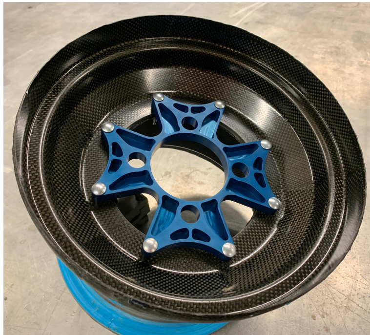
In house manufactured carbon rim after having the wheel center mounting holes drilled
