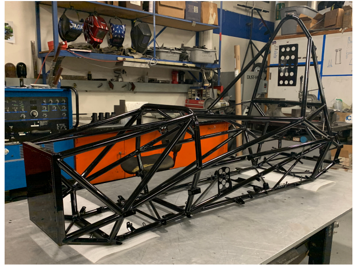
Above: F-20's chassis freshly back from powdercoating Below: Parts laid out after being polished in preparation for anodization
